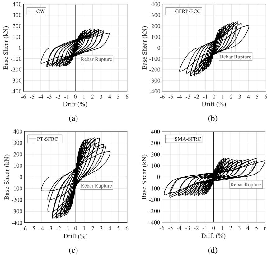
Figure 3. Hysteretic responses of specimens: (a) CW, (b) GFRP-ECC, (c) PT-SFRC, (d) SMA-SFRC.
