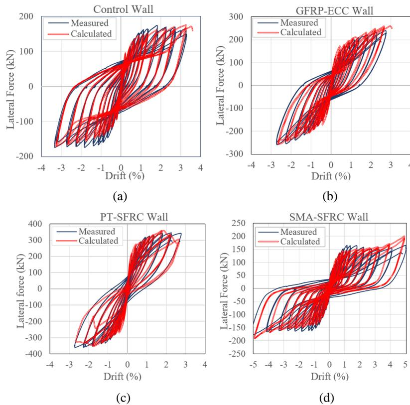
Figure 5. Calculated and measured hysteretic responses specimens: (a) CW, (b) GFRP-ECC, (c) PT-SFRC, (d) SMA-SFRC.
