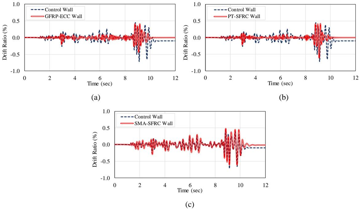
Figure 7. Response histories of the innovative specimens vs. the control wall: (a) GFRP-ECC, (b) PT-SFRC, (c) SMA-SFRC.
