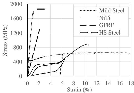
Figure 2. Stress-strain relationships of reinforcing materials.
